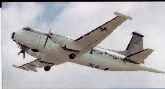
Above: One of Germany's Atlantics shows its retracted radar radome and sonobuoy launch tubes.
